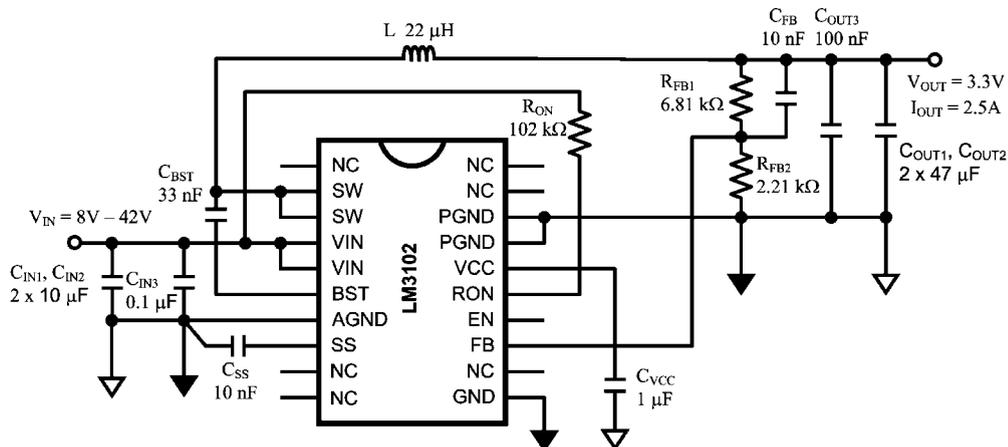
Typical Application Schematic for V<sub>OUT</sub> = 3.3V
