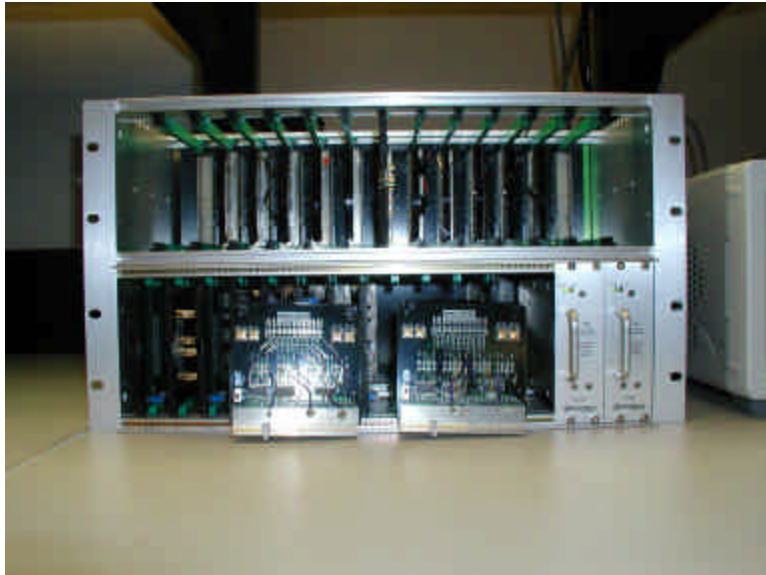
Figure 10 Photo of the evaluation backplane and test boards.
