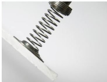
Fig. 3 - Spring after compression; the conical section collapses to form an electrode disk.
