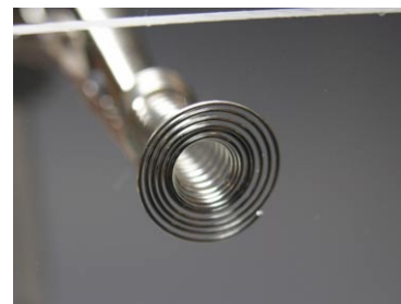
Fig 4 - Compressed spring, viewed from front through a clear panel. The channel in the middle can be used for an LED (as with the S-presso).
