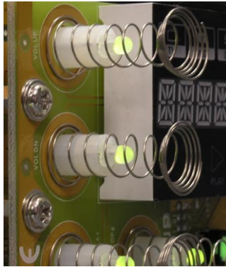
Fig. 5 - Asus S-presso uses Philipp™ springs attached to LED mounts to bridge the air gap to the panel and to simultaneously allow key backlighting.
