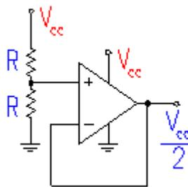
An easier way to do this is to use a virtual ground circuit, such as the [TLE2426](#) virtual ground (the "Rail Splitter") from [Texas Instruments](#). It generates an output precisely midway between the two supply rails, has noise reducing circuitry and can source and sink about 20 mA. You can also find these in the lab.
