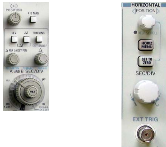
Figure 2: Typical horizontal (timebase) control of an analog (left) and digital oscilloscope (right).
