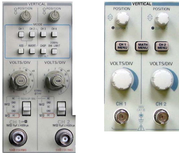
Figure 1: Typical vertical gain controls of a two-channel analog (left) and digital oscilloscope (right).
