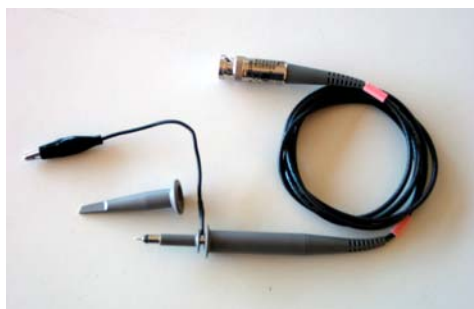
Figure 4: a) A scope probe;
