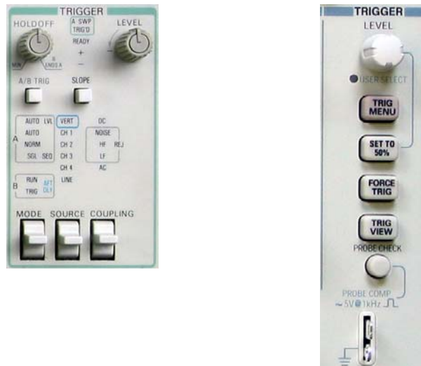
Figure 3: Typical trigger controls of an analog (left) and digital oscilloscope (right).
