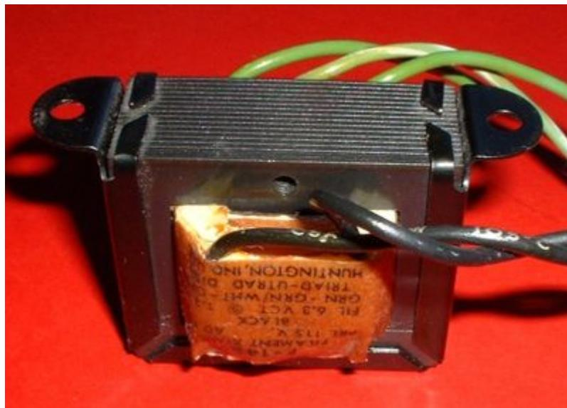
current heating of the core. The thin laminations are used to reduce the eddy currents, and the insulation is used to keep the laminations from acting as a solid piece of steel. The thinner the laminations, the lower the eddy currents, and the lower the losses. Very thin laminations are generally used on high frequency transformers. The cost goes up when using thinner laminations mainly over the labor in stacking them.
