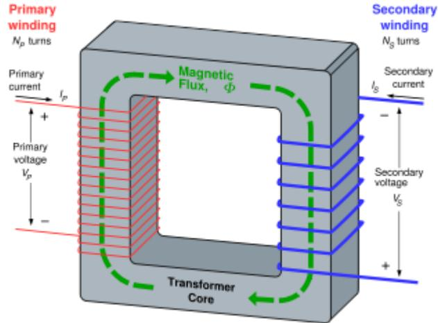
MMF produces a varying magnetic flux  $\Phi_P$  in the core, and, with an open circuit secondary winding, induces a back electromotive force (EMF) in opposition to  $v_P$ . In accordance with Faraday's law of induction, the voltage induced across the primary winding is proportional to the rate of change of flux:
