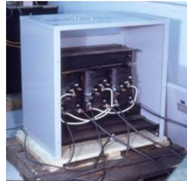
Experimental power transformers in the 2 MVA range have been built with superconducting windings which eliminates the copper losses, but not the core steel loss. These are cooled by liquid nitrogen or helium.
