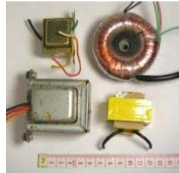
Ferrite toroid cores are used at higher frequencies, typically between a few tens of kilohertz to a megahertz, to reduce losses, physical size, and weight of switch-mode power supplies.
