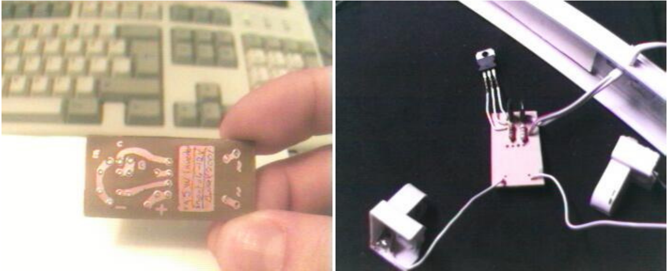
Etched PCB and PCB with components mounted on, without transformer
