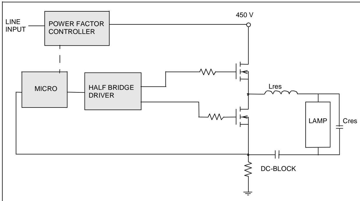
In this diagram, the microcontroller takes the place of the VCO and the control logic. The microcontroller has an output(s) that emulates the VCO output which in turn controls the turn-on and turn-off the upper and lower portion of the half bridge. In this manner, the dead time, frequency, and duty cycle of the half bridge output can all be independently controlled.
