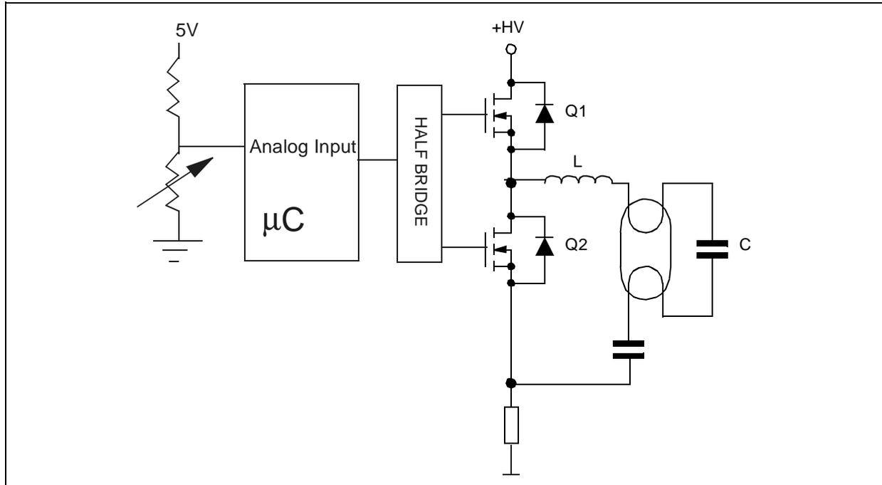
When a pin is configured as an “analog input” it acts as an A/D converter and looks at the voltage on the pin and transforms that voltage of 0V to 5V into a corresponding number between 0 and 255. For example, if the voltage on the Analog Input pin is 2.5 V, then the A/D will convert the 2.5V to a value of 128. The program that has been stored in the micro may then in turn tell an output pin to change the frequency of the half bridge to that of a 50% dimming level.
