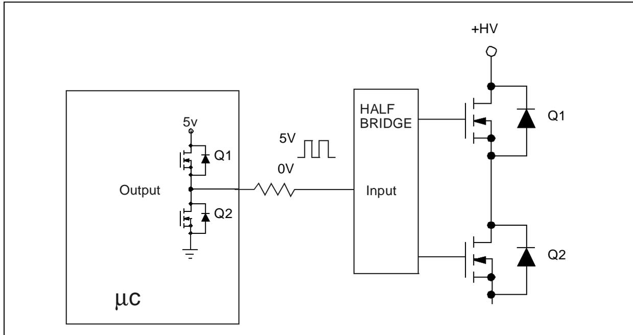
In this example, the pin is configured as a push-pull output. The output pin goes from a “low” to a “high” state, which in turn applies 0V on the output pin and then 5V correspondingly. A “low” on the pin is accomplished by turning on the lower FET in the  $\mu\text{C}$ , thus pulling the output pin to ground. A “high” is accomplished by turning off the lower FET and turning on the upper FET in the microcontroller.
