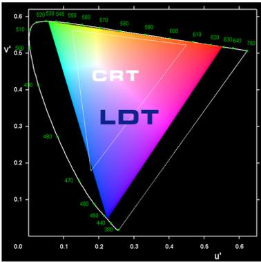
Fig. 2: The “corners” (primary valencies) of the laser color triangle of LDT are in singular value wavelengths, that is pure, unmixed colors of high saturation compared with other projection technologies such as CRT projectors.
