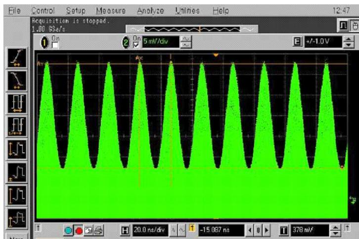
Fig. 5: Test showing the real column contrast of an LDT projector. The difference in luminous density is more than 50%.
