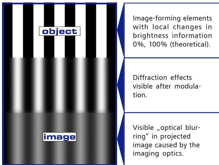
Fig. 4: The optical transfer function of conventional projection methods reduces the actual resolution considerably.
