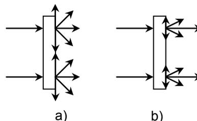
Fig. 10 a) diffuse screen; b) gain screen
