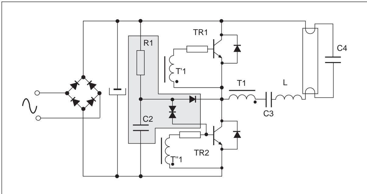
Figure 3. Start-up of the voltage fed ballast
