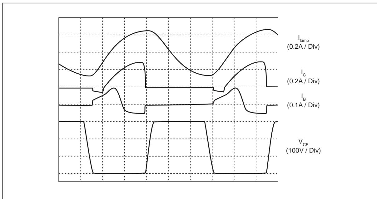
20V above the nominal value of 120V RMS and no lamp connected in a), and "arcing" testing of the ballast during installation in b). Figure 7a shows that the  $V_{CE}$  of the transistor can reach around 600V,
